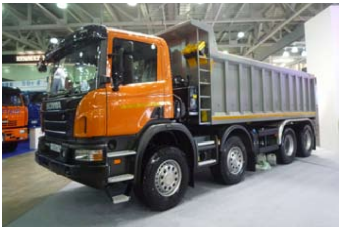
Самосвал Scania P440 8x4 Off-Road
